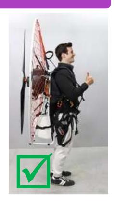
For a correct posture of the paramotor which must not be too close to the head nor too low to touch the legs, it is necessary to act on the shoulder strap adjustment by pulling or loosening them enough to obtain the right position.
