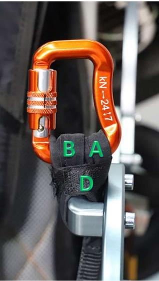
Once the carabiners have been assembled, check for correctness angle them so that they are both facing forward, as indicated below, to facilitate the pilot during take-off, landing and exiting the harness.
