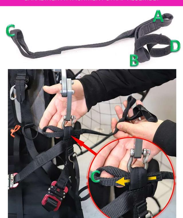
To correctly assemble the carabiner attachment strap, first insert the end "C" in the loop of the harness belt hooked to the shackle.
