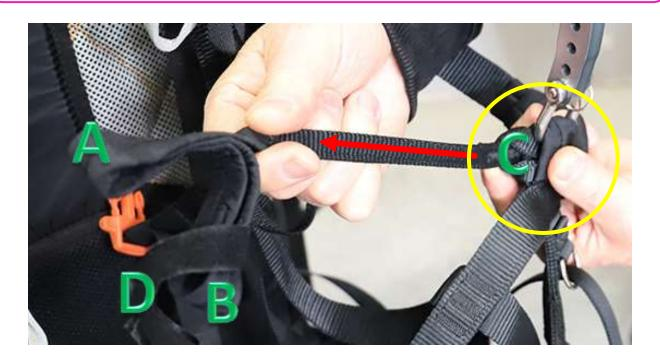
pass side "A" into the carabiner loop attachment on the pivot arm and lift loop "B" until it matches loop "A"
