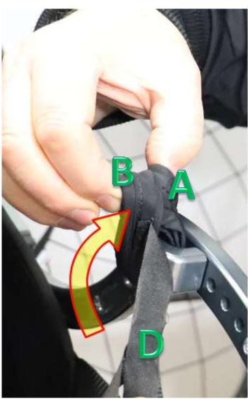
Insert the carabiner into the loops "B" and "A" so that by rotating it remains in position with the closure facing the pilot.
