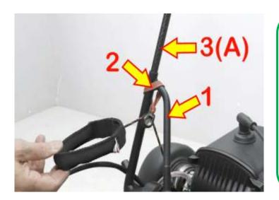
**To start:**Insert the starter support "D" on the central engine frame first.
