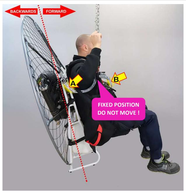
If the paramotor is tilted too far back it means that the pilot is light compared to the spacer adjustment,
