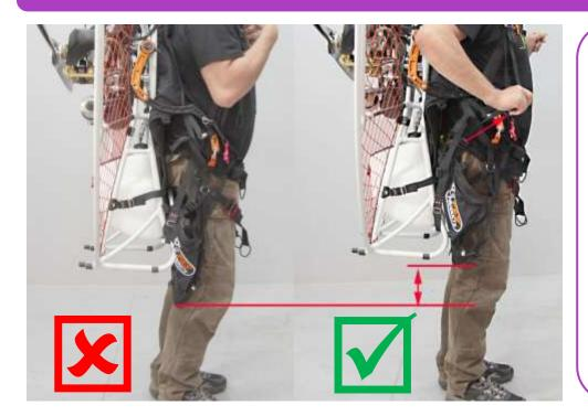
Harness height adjustment to facilitate the takeoff run.
