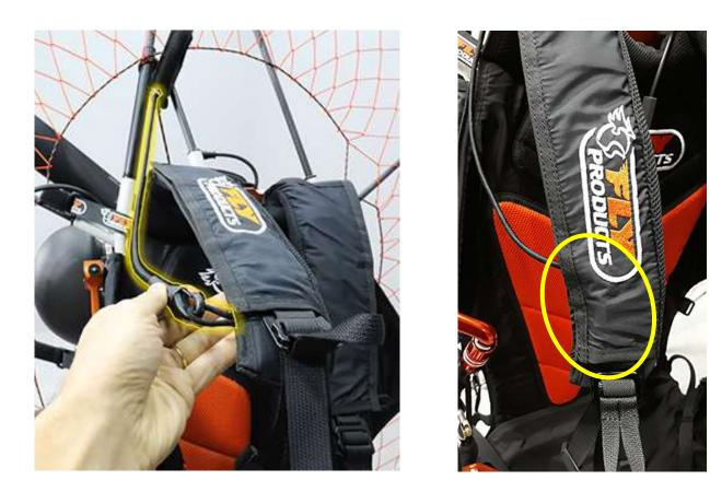
Hook the elastic rope of the starter handle to the prepared eyelet and lock it under the velcro for 5-10 cm. (2-4 In.)
