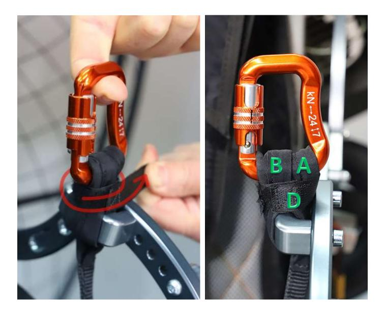
Once the carabiners have been assembled, check for correctness angle them so that they are both facing forward, as indicated below, to facilitate the pilot during take-off, landing and exiting the harness.
