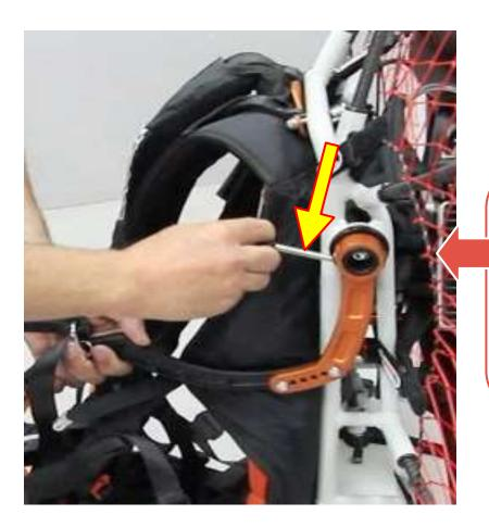
Put the pivotarms in position and, taking care to keep the holes in axis, block them with the push pins. CHECK THAT THEY ARE LOCKED!
