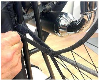
Pull the velcro until you have the maximum tension of the net.
