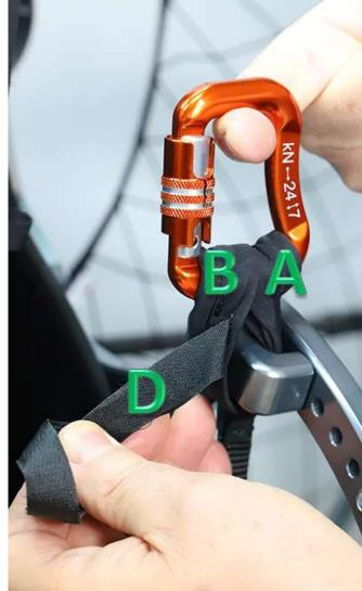
To finish assembly, wrap very tightly velcro "**D**" around loops "**B**" and "**A**" so that the carabiner remains in the correct position.
