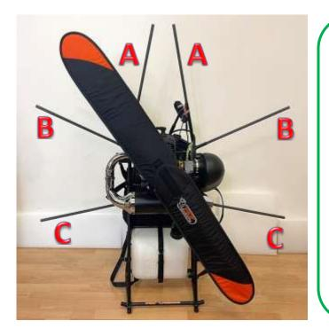
Complete the insertion of the rods according to the length, as previously indicated, in the appropriate housings:
