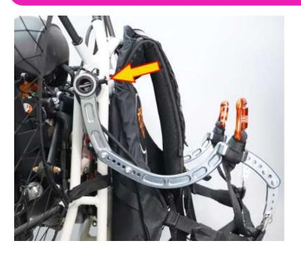
Install the pivot arms in position and, taking care to line the holes, lock them with the push pins keeping the button pressed and releasing it only after it has completely entered. Make sure the pushpin is secured.
