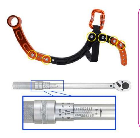
Do not over tighten these nuts to avoid weakening the structure and therefore the seal! Preferably use a torque wrench calibrated at **10** N-m (Newton / meter) which correspond to about **1** Kg. (**2.2** lb)
