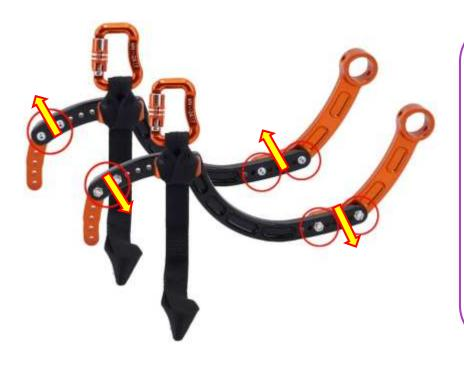
The first rule to be observed is the position of the attachments according to the direction of the fixing screws. The bolt heads are positioned inside and the nuts on the outside of the arms, this to avoid wear of the harness by rubbing the parts.
