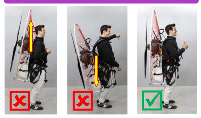
For a correct posture of the paramotor which must not be too close to the head nor too low to touch the legs, it is necessary to act on the **shoulder strap** adjustment by pulling or loosening them enough to obtain the right position.
