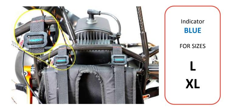
Hook the lower harness anchoring straps taking care to pass behind the leg of the frame and then under the lower bar as shown in the photo.
