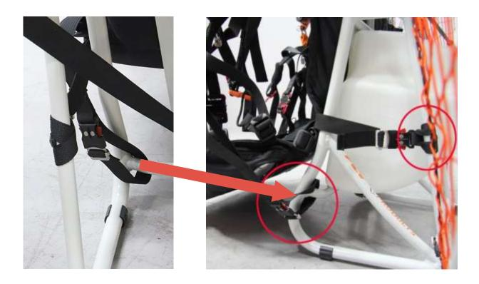
Lock the four lower straps onto the quick-lock bucklets.
