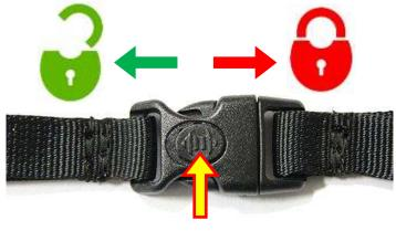
Lock the coupling by moving the button as shown in the figure.
