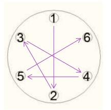
Screw all the propeller bolts without forcing. Tighten them gradually following the correct sequence as indicated.
