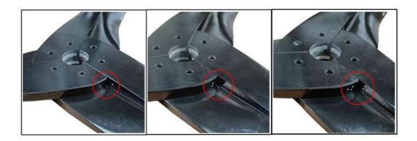
When assembling the three-blade propeller, pay close attention to the sequence indicated on the back of the propeller
