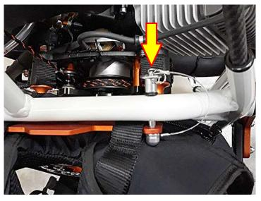
Insert the harness on the harness plate and lock the push-pin.
