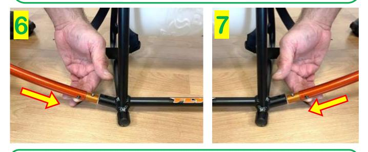
Then proceed to the RIGHT and LEFT lateral connection of the two lower and upper semicircles, checking that the sealing button has come out correctly from its hole and that the part is actually locked.
