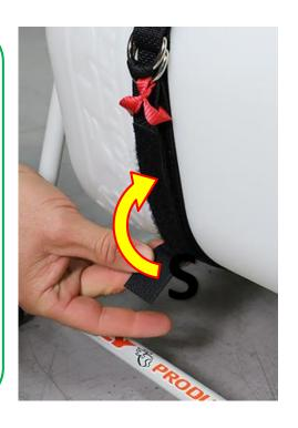
To release the tank, open the safety little belt (S), detach the velcro from the closure, release the red eyelet and pull it back to help the rings open.
