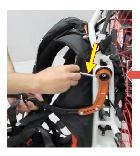
Put the pivotarms in position and, taking care to keep the holes in axis, block them with the push pins.
