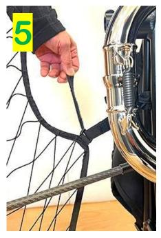
Unlock and release the net from the RIGHT and LEFT side velcro straps, taking care to close the velcros on itself.
