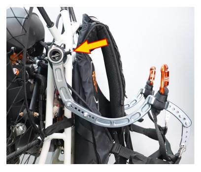
Install the pivot arms in position and, taking care to line the holes, lock them with the push pins keeping the button pressed and releasing it only after it has completely entered.
