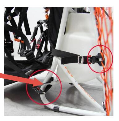
Lock the four lower straps onto the quick-lock bucklets.
