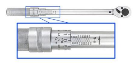
Do not over tighten these nuts to avoid weakening the structure and therefore the seal! Preferably use a torque wrench calibrated at 10 N-m (Newton / meter) which correspond to about 1 Kg. (2.2 lb)
