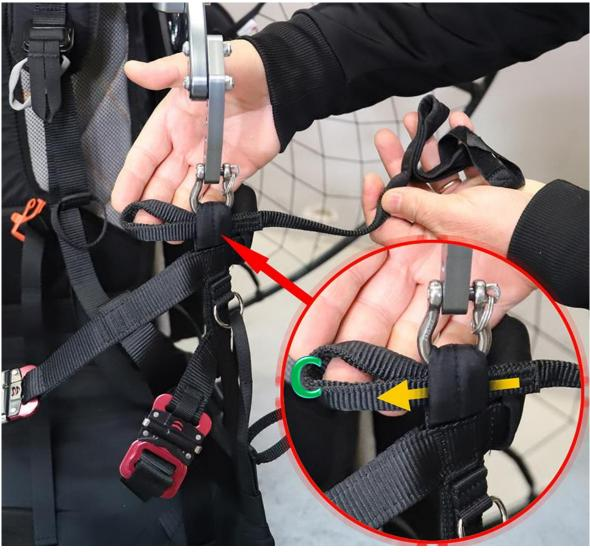
To correctly assemble the carabiner attachment strap, first insert the end "C" in the loop of the harness belt hooked to the shackle.
