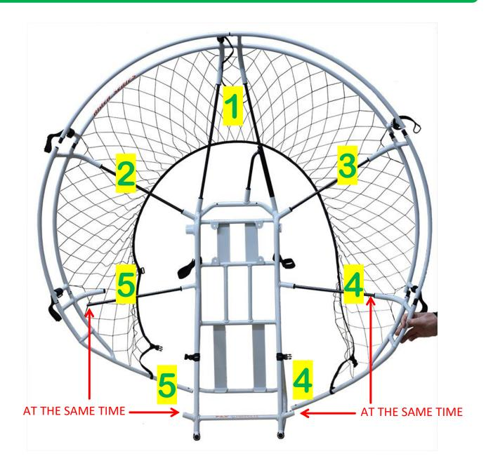
In order not to force the net excessively, it is recommended follow the illustrated sequence with the parts **DETACHED** from each other taking care to insert points "4" AT THE SAME TIME and finally again at the same time points "5" making sure the snap pins are perfectly inserted.
