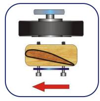
Propeller mounting on motors with **BELT reduction** (COUNTERCLOCKWISE ROTATION) for the **MOSTER** engine.
