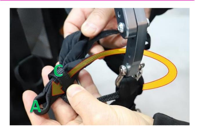
When all the strap has passed, tighten the loop that has formed around the harness belt loop by pulling the extremity tightly and adjusting it with your fingers.
