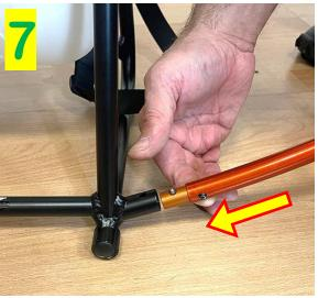
Then proceed to the RIGHT and LEFT lateral connection of the two lower and upper semicircles, checking that the sealing button has come out correctly from its hole and that the part is actually locked.
