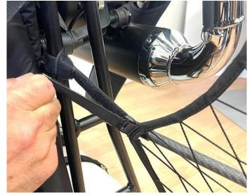
Pull the velcro until you have the maximum tension of the net.
