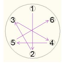
Screw all the propeller bolts without forcing.
