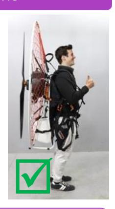
For a correct posture of the paramotor which must not be too close to the head nor too low to touch the legs, it is necessary to act on the **shoulder strap** adjustment by pulling or loosening them enough to obtain the right position.
