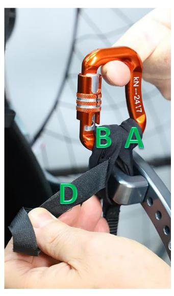
To finish assembly, wrap very tightly velcro "D" around loops "B" and "A" so that the carabiner remains in the correct position.
