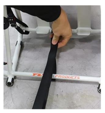
Turn the strap around the tube between the two velcroes, and close them to stop it. Place the tank in the correct position onto its supports and lock it as shown below.
