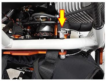
For a correct use of the push-pin, keep the button pressed while inserting and while closing the safety cap,
