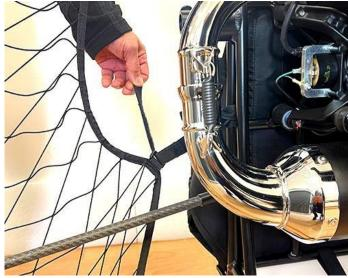
Open the velcro and pass it through the prepared eyelet following the direction indicated.
