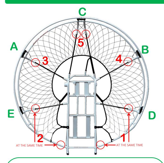
For disassembly, after opening all the closing velcro straps,
