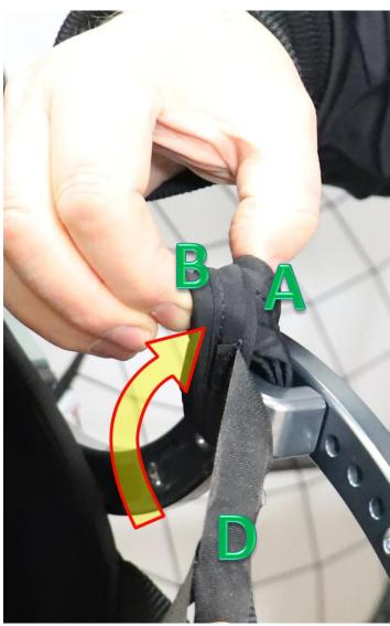
Insert the carabiner into the loops "B" and "A" so that by rotating it remains in position with the closure facing the pilot.
