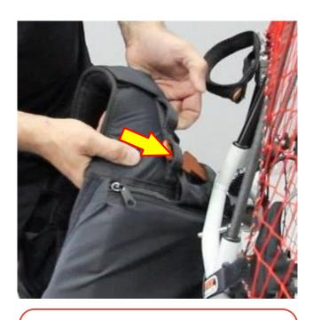
Insert the harness on the harness plate and lock the push-pin.
