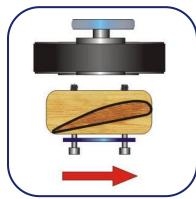
Propeller mounting on motors with **mechanical reduction** (CLOCKWISE ROTATION) for the **ATOM** and **THOR** engine.
