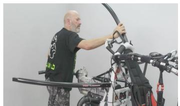
Lock the arms with the safety velcro taking care to insert the pins in the appropriate holes
