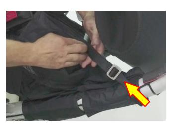
Position of the elastic safety hook and the velcro hook (in yellow) to engage the kill switch device (in red)
