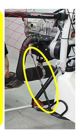
If a ballistic emergency parachute is installed, pass the rubber band behind the emergency belt into the appropriate eyelet.
