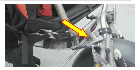
position the leg and screw the bolt, WITHOUT LOCKING for now, beginnings from the front support
