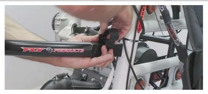
Pass the belt in the buckle, tension and go back by locking the velcro on itself
