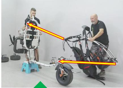
Place the rear part on a support about 30 cm high and raise the motor base vertically
