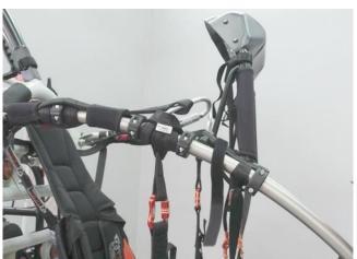
First tighten the screws on both sides and then close the velcroes
