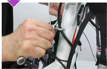
The emergency belt is already wired on the motor support, hook the two ends to the karabiners and lock them on the cradle with the apposite elastic velcroes
