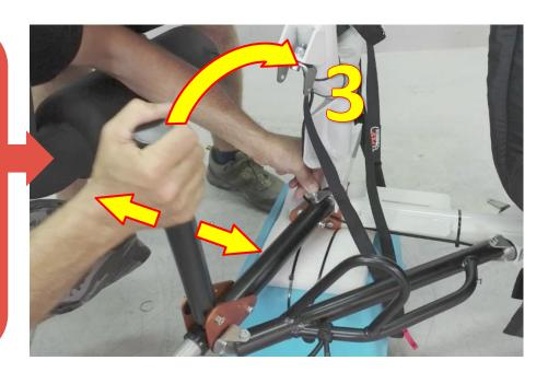
position and lock the upper bolt and the two other bolts, repeat the same operations for mount the other leg
