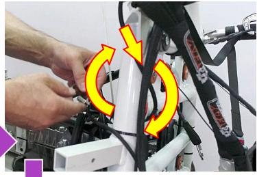
Wrap one end of the safety wire around the frame tube, hook it onto itself and lock the hook.
