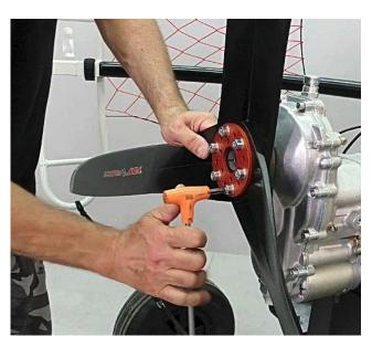
Assemble the propeller covers starting from the one with the belt on the tip, then placing the blade in a vertical position
