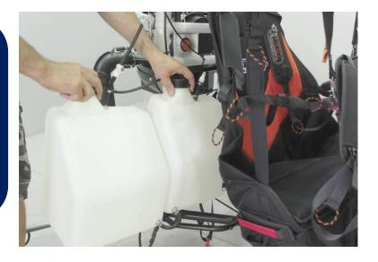
Block the tanks with a double turn of the belt on the frame
