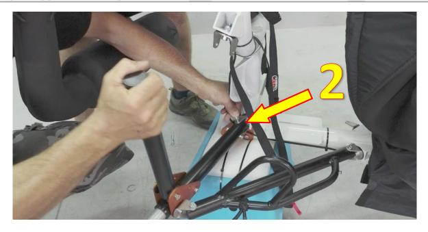
Move the third support slightly to center the clutch on the frame
