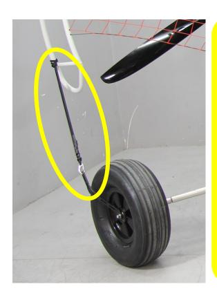
Hook the elastic bands down to the prepared connections
