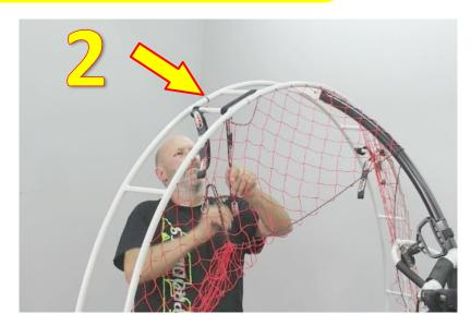
Lock the arms side with the safety velcro taking care to insert the pins in the appropriate holes
