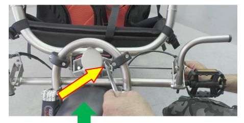
position and lock the bolts on the lower side
