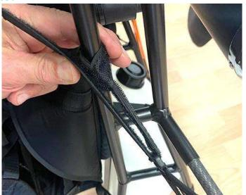
Lock the velcro in correct position by pressing it on the underlying loop.
