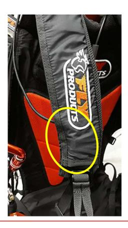
Hook the elastic rope of the starter handle to the prepared eyelet and lock it under the velcro for 5-10 cm. (2-4 ln.)
