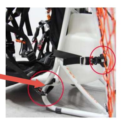
Hook the four lower straps onto the quick-lock provided bucklets.
