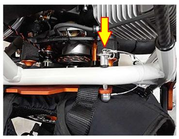
For a correct use of the push-pin, keep the button pressed while it is slipping and while closing the safety catch,
