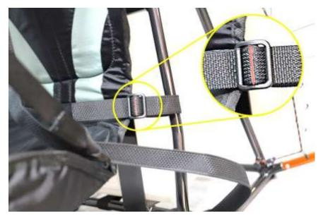
Hook the middle side straps of the harness having as a reference the red seam as shown in the photo.
