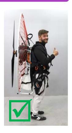
Adjust the vertical position of the paramotor on the shoulders.
