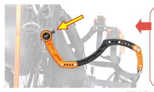
Put the pivot arms in position and, taking care to line the holes, lock them with the push pins keeping the button pressed and releasing it only after it has completely entered.
