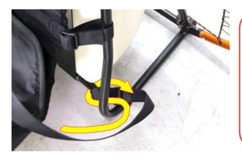
Hook the lower harness anchoring straps taking care to pass behind the leg of the frame and then under the lower bar as shown in the photo.
