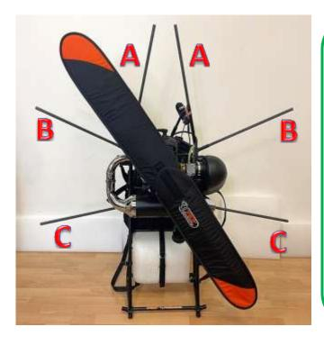
Complete the insertion of the rods according to the length, as previously indicated, in the appropriate housings:
