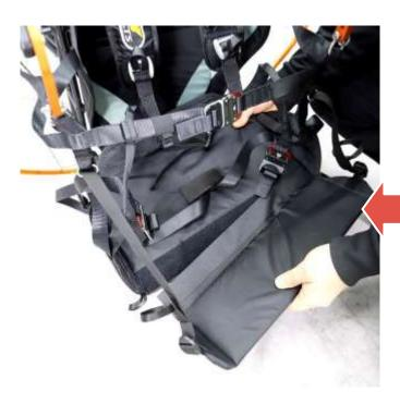
It is possible to adjust the seat deep by removing or adding the extension blocking it on the prepared velcro.
