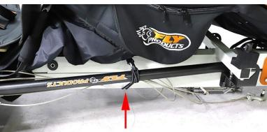
Then lift the cradle and raise the paramotor's coupling support in a vertical position, join the cradle to the support using the special butterfly screw:
