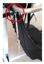
Start with the right rod locking it with the push-pin and then hook the left tie-bar tightening the lever until the holes to be fitted match the push-pin
