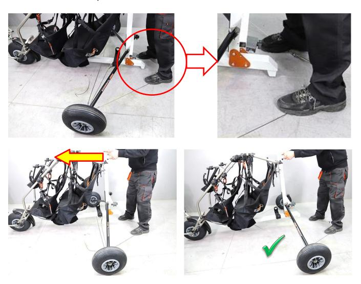
Lock the wheels in place using the lower tie-rod with the elastic:
