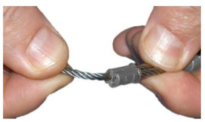
Check the wear and the oxidation conditions of the steel cables of the rear wheels, if they are not in good condition, do not hesitate, replace them immediately!
